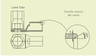
The dimensional stability in diameters with strict tolerances either inside or outside of the barrel, ensures the correct fixation and repeatability in the quality of the hexagonal indentation or compression, in this case, permitting the use of defined matrix. The entrance of the conductor is easier with the corresponding chamfer.
